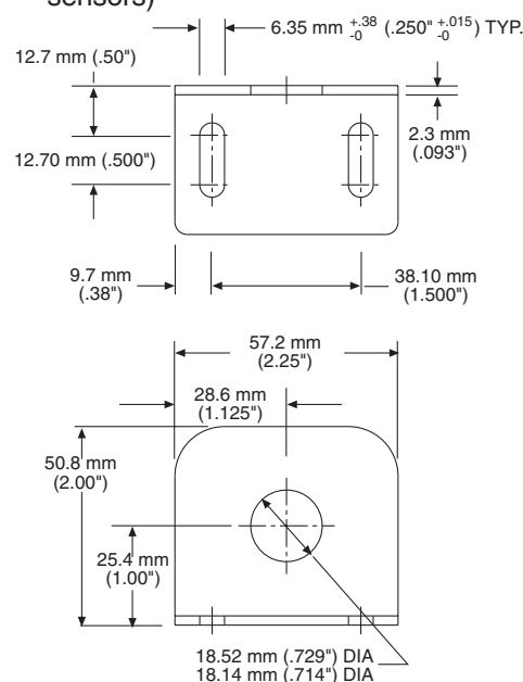
**AC228** Small, right-angle, stainless, mounting bracket (for 18 mm barrel sensors)
