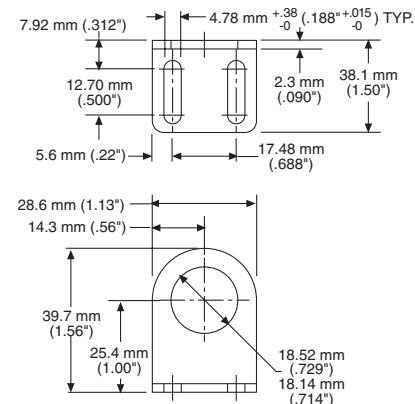
**AC231** Straight, stainless mounting bracket (for flat-profile sensors)
